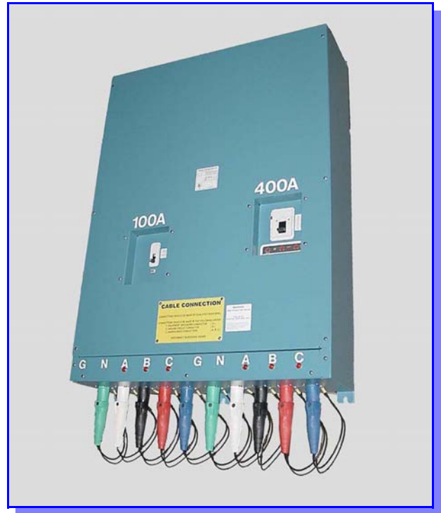
CSDC-60B4121-SC Custom 600A. Dual Breaker Company Switch 600A. Bus, (1) 400A., (1) 100A. Branch with SafeCam® Outlets
